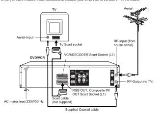
In addition to the coaxial cable connection, you should also connect the SCART cable from the DVD/VCR to your TV as shown. As well as transferring the high quality pictures and sound to your TV, the SCART connection can automatically switch the TV to its AV channel for playback.
